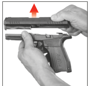
Figure 25 Lifting the slide from the frame
