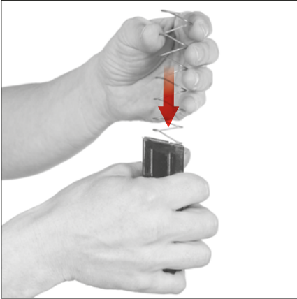
Figure 44 — Insert the follower and spring
