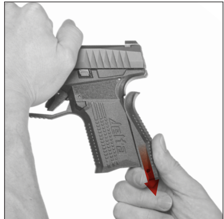
Figure 9 — Removing/installing the backstrap
