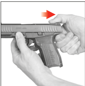
Figure 23 Pulling slide back slightly and holding it
