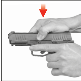
Figure 42 Placing the slide on the frame (note slide is slightly forward in regard to its closed position)
