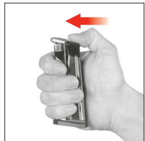
Figure 12 Emptying the magazine
