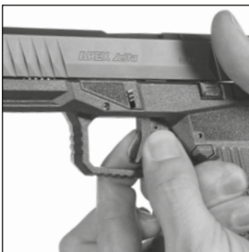
Figure 51 Checking the trigger safety - trigger should not move rearward under pressure if the safety latch is not depressed
