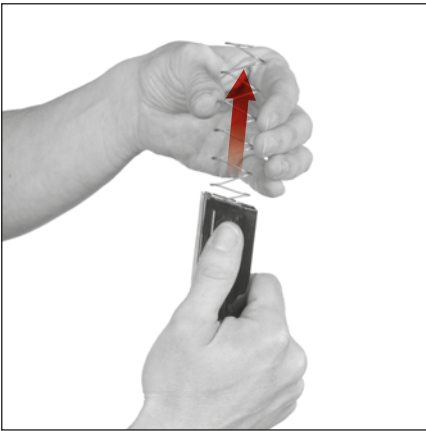
Figure 30 — Removing the spring with follower
