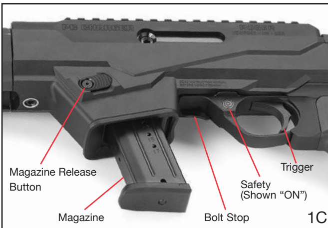
Figures 1A, B, C. In these illustrations the frequently used operating components are identified. Note that the safety is fully depressed into the left side of the trigger guard (and fully protruding from the right side, which is not visible) and is therefore in its "ON" (safe) position.
