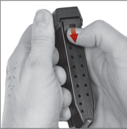
Figure 32 — Pulling on the locking plate tab to free the floorplate
