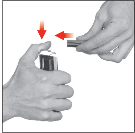
Figure 45 — Compress the spring into the magazine body while sliding the floorplate onto guides
