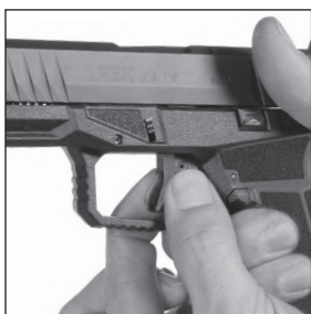
Figure 51 Checking the trigger safety - trigger should not move rearward under pressure if the safety latch is not depressed
