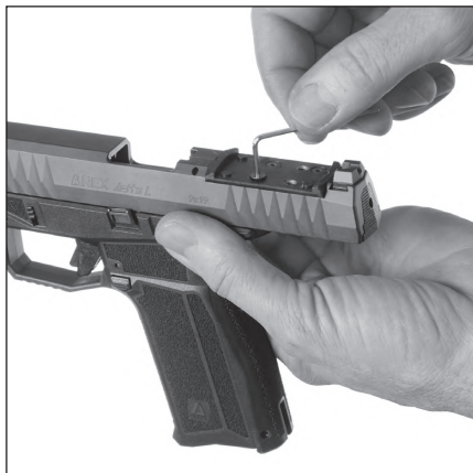
Figure OR6 - Mounting the appropriate interface plate
