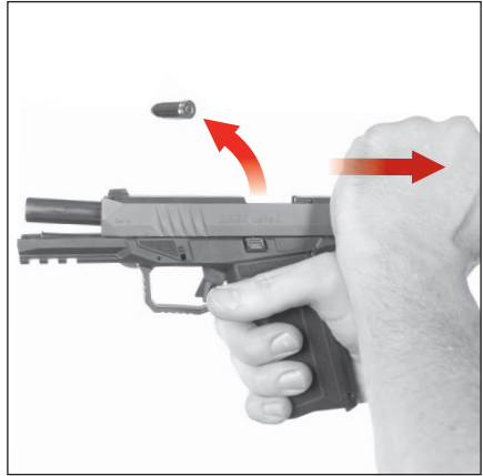
Figure 5 — retract slide: watch for ejected cartridge
