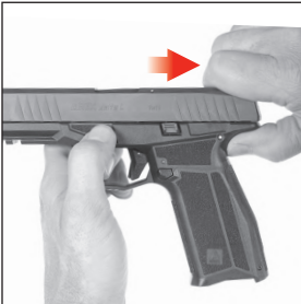
Figure 23 Pulling slide back slightly and holding it
